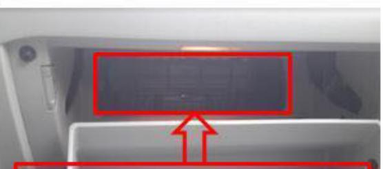
FILTER IS INSIDE THIS CASE. INSTALL NEW FILTER HERE.
