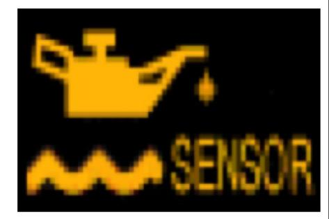
OIL LEVEL LOW OR OIL PRESSURE LOW: Low engine oil level or low pressure level can lead to internal damage of engine and its components. Get assistance immediately. Don't drive vehicle until resolved.
